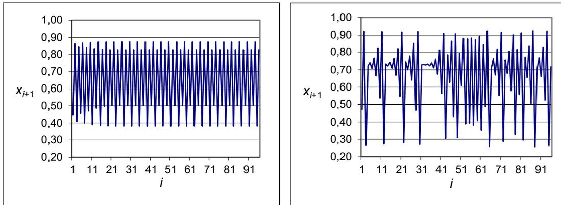
Figure 2: The graph of logistic function with parameters  $x_0 = 0.85$  and  $r = 3.5$  or  $3.7$
