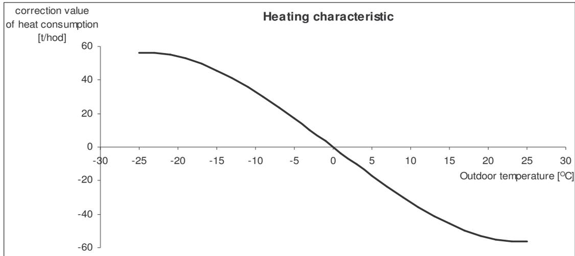
Fig. 6: The sample of heating characteristic (cubic function)
