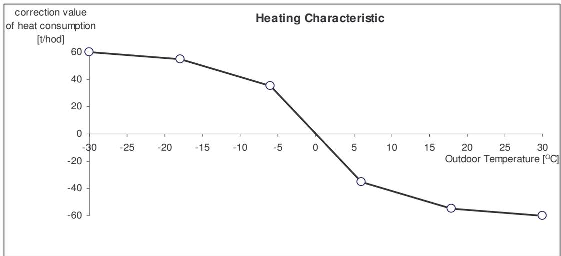
Fig. 7: The sample of heating characteristic (piecewise linear function)
