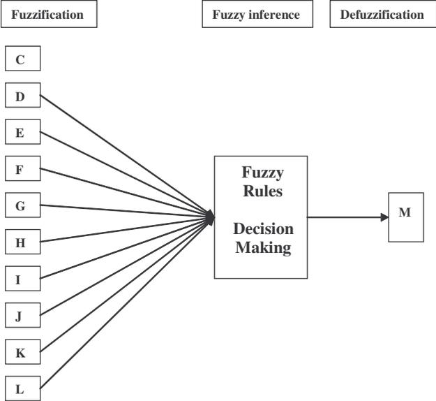
Fig. 2. Scheme of fuzzy logic decision making process
