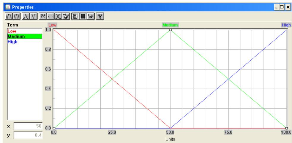
Fig.3. The attributes and membership functions of variable Properties
